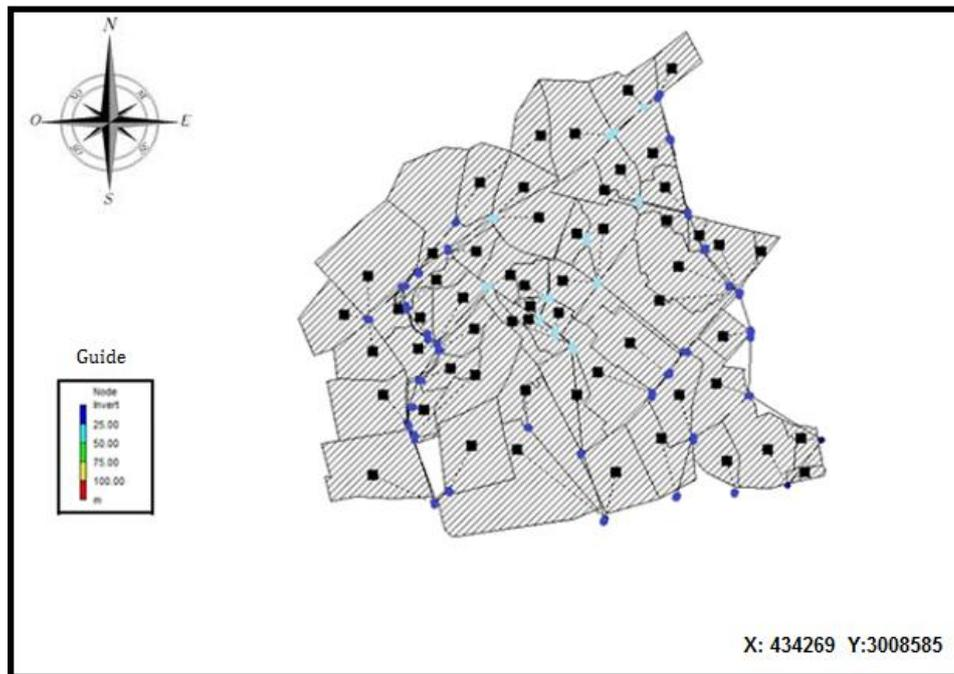
**Figure 1.** The amount of water overflow in the joints obtained from SWMM software
