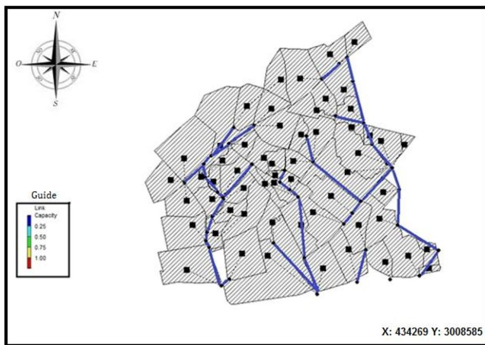
**Figure 2.** Discharge capacity of the channels obtained from SWMM software
